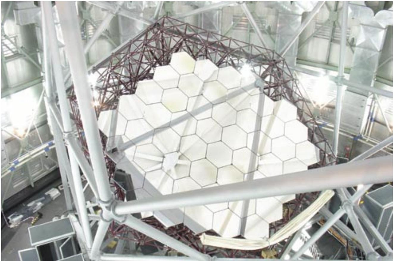
Figure 10. 51 installed mirror segments in SALT (October 2004)
